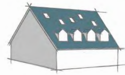
Large roof to wall ratio, excessive amount of dormers and skylights
