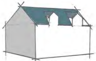
Dormer windows extending upwards out of main walls
