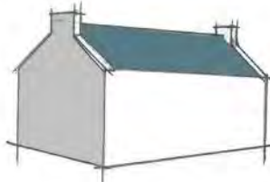
Simple gable roof
