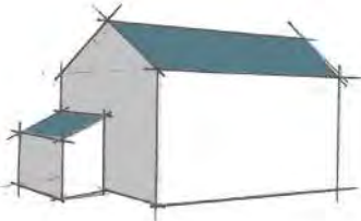
Simple gable roof and tin/slate lean to
