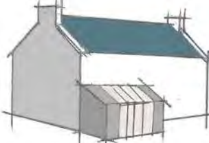
Rear lean to extension with large openings
